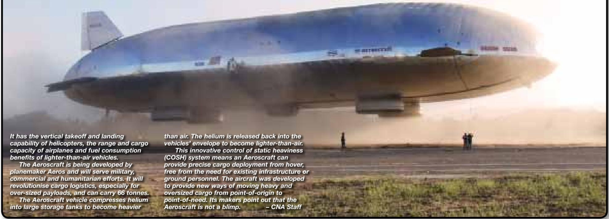
It has the vertical takeoff and landing capability of helicopters, the range and cargo capacity of airplanes and fuel consumption benefits of lighter-than-air vehicles.
