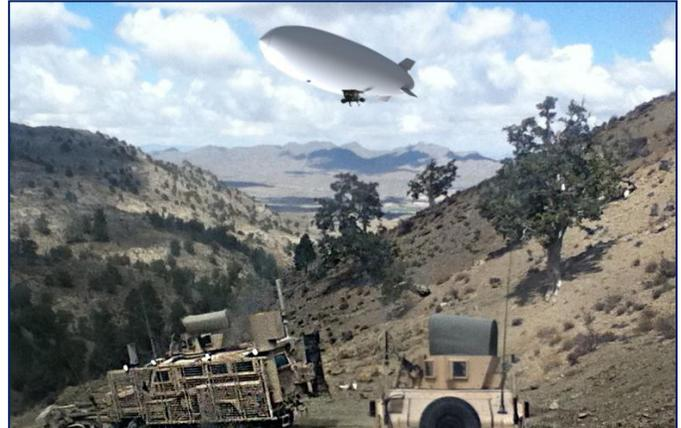
The design provides customers in excess of one ton of useful payload capability and flexibility, as well as improved operational safety and reduced ground handling requirements. Propulsion advancements include ‘vectored thrust’ capability and control, provided by two rotating 4-cylinder engines, coupled with an electronic fuel injection system to improve fuel economy. Controllable-pitch engines enable the 40E to land on shorter fields with reduced speed and angle of attack.
