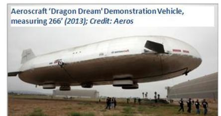
The Aeroscraft is a new heavy-lift, variable-buoyancy cargo airship featuring an onboard buoyancy management system, rigid structure, vertical takeoff and landing performance, and operational abilities at low speed, in hover, and
