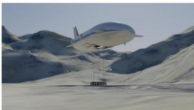
from unprepared surfaces. The discriminating military utility in the Aeros technology approach is VTOL and hover capability at max payload without the use of off-board ballasting, and off and on-loading payloads while hovering; this capability is unique to the Aeroscraft and enabled by Aeros’ Patented control-of-static-heaviness (COSH) onboard buoyancy management technology. This new
