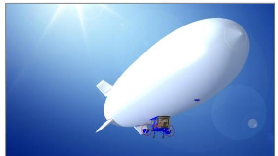
station and operational cost advantages when delivering 360° perspective of the air and ground environment, Aeros' long-loitering 40E airship features useful payload greater than one ton, and supports ISR mission success and efficiency with multi-payload mounting systems for radar, EO/IR cameras, remote sensing technology (LIDAR), and/or communications equipment. It has the following performance characteristics:
