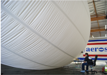
Pressure testing the 40E aft ballonet following assembly
