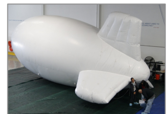
Workers inspect Aeros’ Tactical-130 Aerostat during a pressure test (2015)
