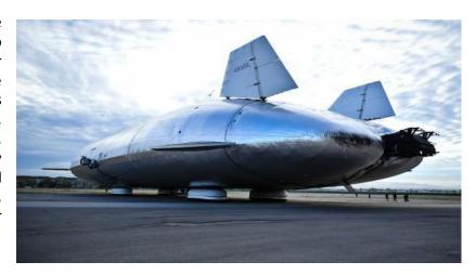
As a result of 4 years of research and development, as well as the success of the first generation Aeroscraft, Aeroscraft Gen 2 will have enhanced buoyancy control, flight surfaces and modular cargo systems. This aircraft will feature zero emission operations, representing the only truly green technology capable of moving cargo over long distances.
